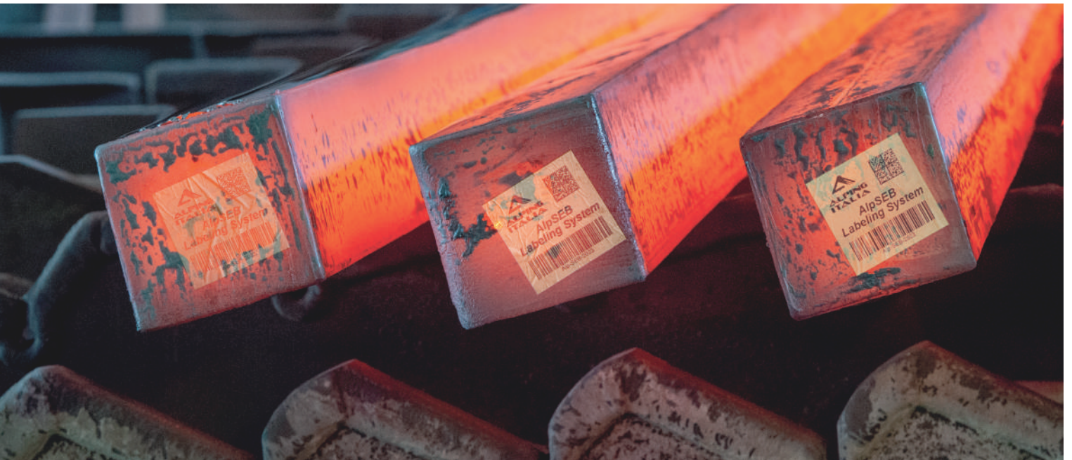
Labels applied to incandescent billets.
